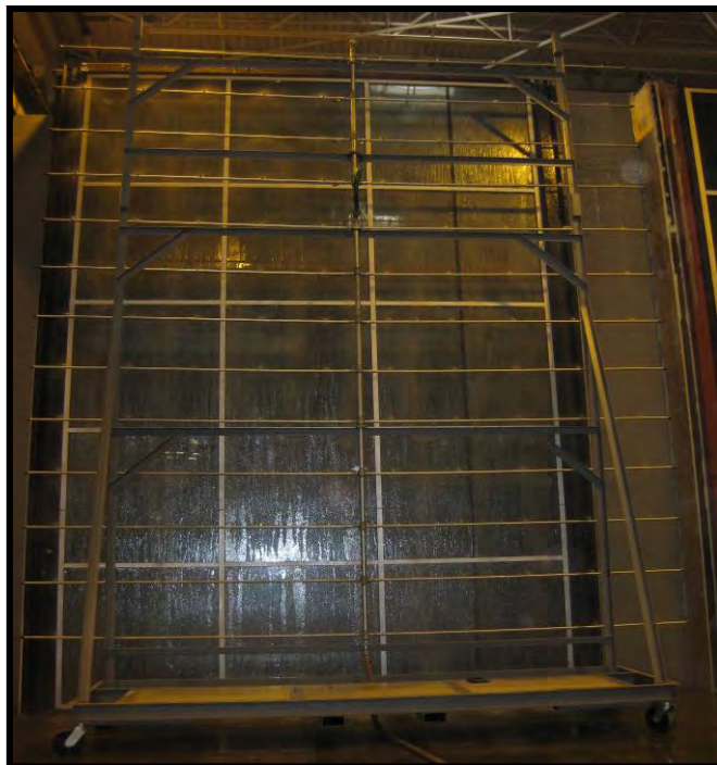
Photo No. 2 Exterior View during Water Penetration Test
