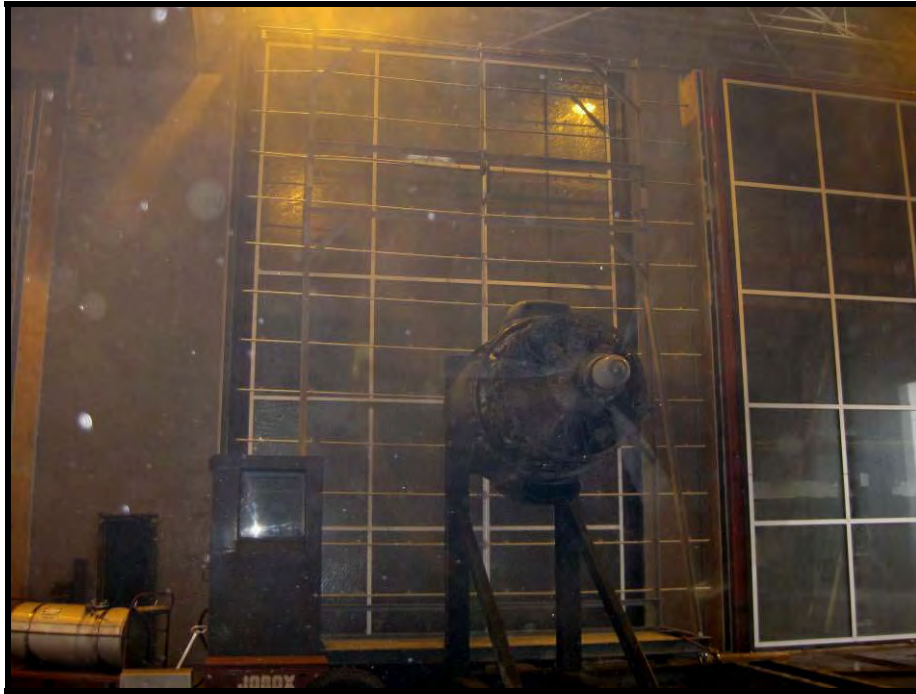
Photo No. 3 Exterior View during Dynamic Water Resistance Test
