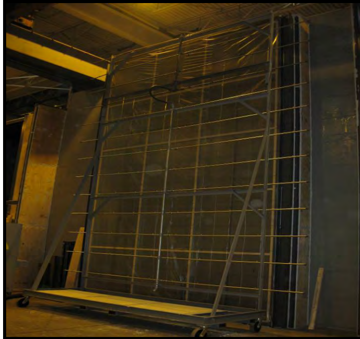
Photo No. 1 Exterior View during Air Infiltration Test
