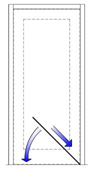
Insert one end of threshold then rotate down until resting on finished floor Fig. 14.1
