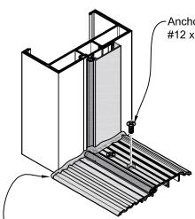
Anchor threshold to clip with  $#12 \times 1/2$ " FH UC.
