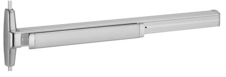
3327A and 3527A for all types of single and double doors, UL listed for panic exit hardware. Devices are ANSI A156.3 – 2008 Grade 1. The 3527A has a smooth mechanism case and the 3327A has grooved case. The surface vertical rod device is non-handed except when the SS (signal switch) option is used. See opposite page for available outside trim and device functions.
