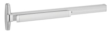
**3349A and 3549A** for hollow metal single and double doors, UL listed for panic exit hardware. Devices are ANSI A156.3 – 2008 (LBL option 2014) Grade 1. The 3549A has a smooth mechanism case and the 3349A has grooved case. The concealed vertical cable device is non-handed except when the SS (signal switch) option is used. See opposite page for available outside trim and device functions.
