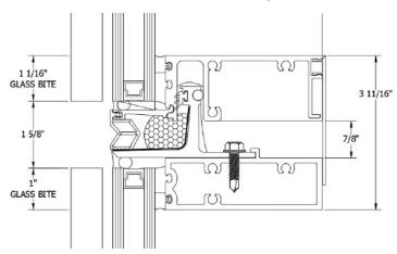
**STARTER SILL** - Allows for quick installation of units with a continuous chicken head at the sill.
