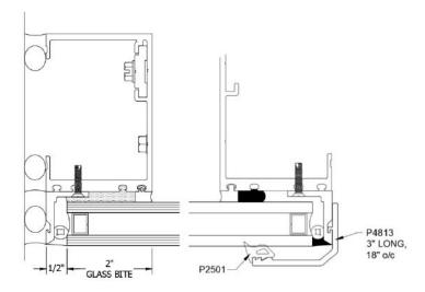
**TEMPORARY SSG RETAINER CLIP** - P4813 integrates with E4212 edge trim to temp the glass during cure.
