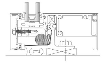
**SSG PERIMETER** - Two options: Glass-to-edge & an applied 7/8" tube.
